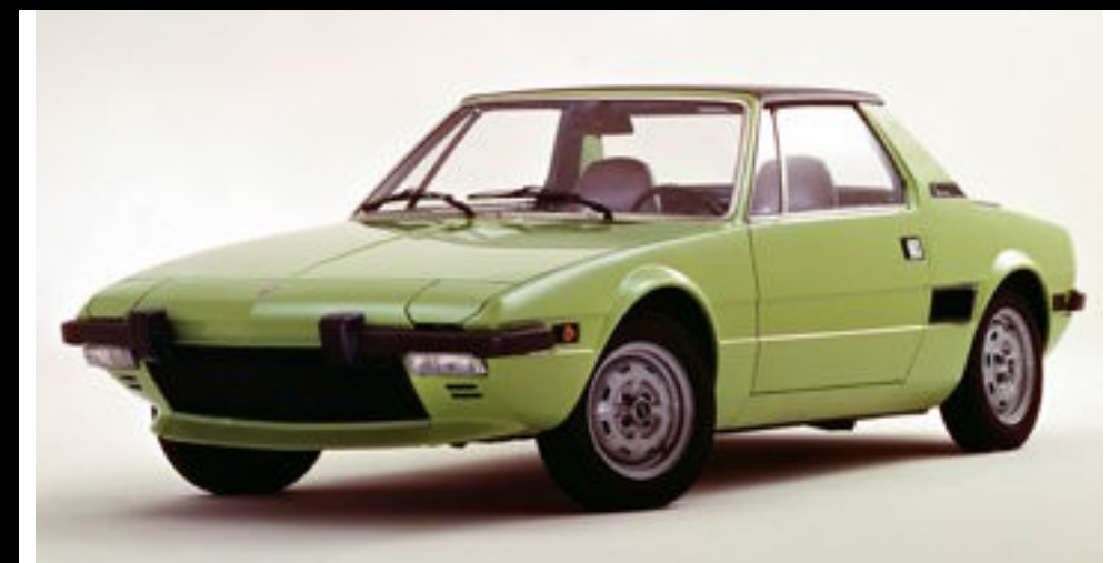
Fiat X 1/9 (1972-1978) Body by Bertone. Featured a new engine position mid-rear and transversal.
